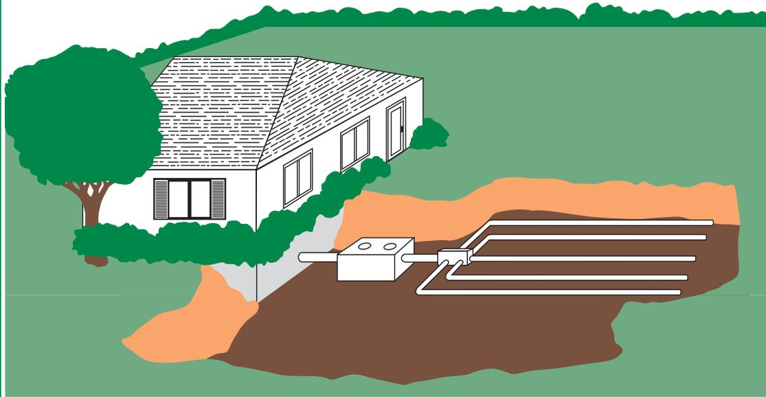
A **septic system** consists of a **septic tank**, a **distribution box** and a **drainfield**, all connected by pipes, called **conveyance lines**.
